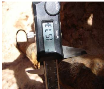
August 2005 - This tower, in Maricopa County, AZ did not collapse. Note that the condition of the anchor shaft at the surface shows no corrosion. Deterioration at two points further down the shaft show significant corrosion.
