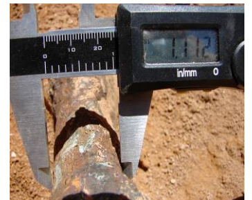
August 2005 - This tower, in Maricopa County, AZ did not collapse. Note that the condition of the anchor shaft at the surface shows no corrosion. Deterioration at two points further down the shaft show significant corrosion.
