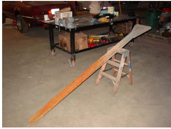
Mitchell - Notice no corrosion until 2' below grade
