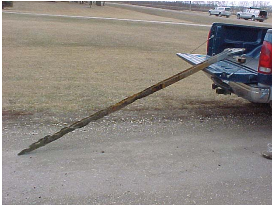
Midwestern United States, March 2003. These pictures are a testimony to the toughness of a guyed tower. Even after the anchor failed holding the top two guy levels although damaged beyond repair the tower remained standing.
