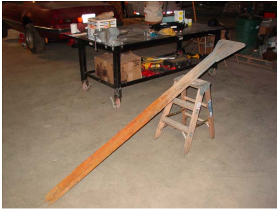
Notice no corrosion until 2' below grade
