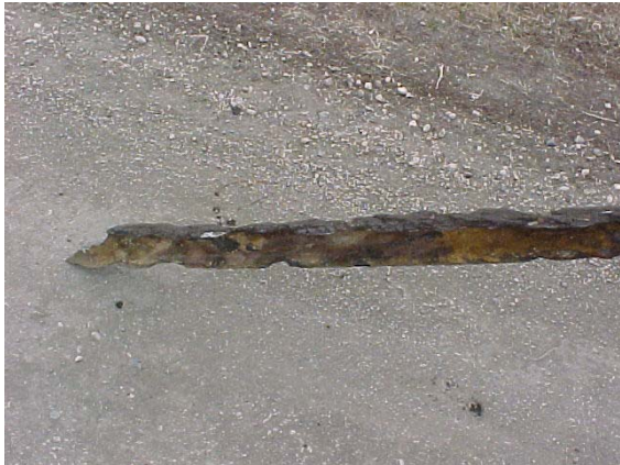
Midwestern United States, March 2003. These pictures are a testimony to the toughness of a guyed tower. Even after the anchor failed holding the top two guy levels although damaged beyond repair the tower remained standing.
