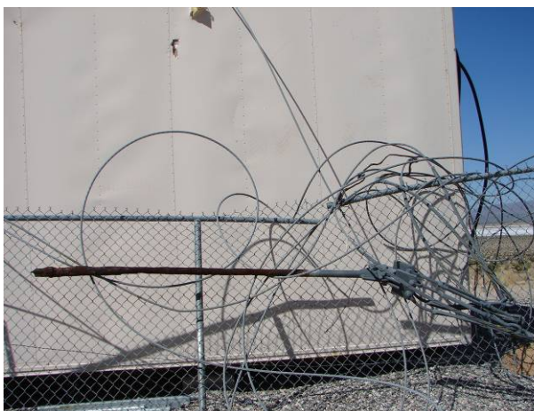
Notice the weakest point was 8 feet below ground level.
