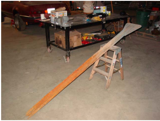
Mitchell - Notice no corrosion until 2' below grade
