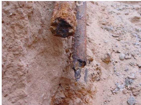
California 1/21/05 – Anchor on temporary chain and close-up of corrosion at break. Note the dry sanding conditions. Dry climates do not preclude active corrosion cells.
